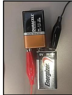
Figure 7. Two 9 V batteries connected in series.
