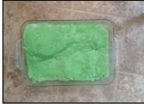
Figure 12. Non-conductive 'waste rock' is added to fill the rest of the container.
